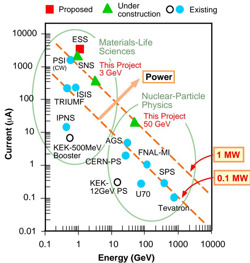
FIG 1.1: Beam energy, beam current, and beam power of world's proton machines
