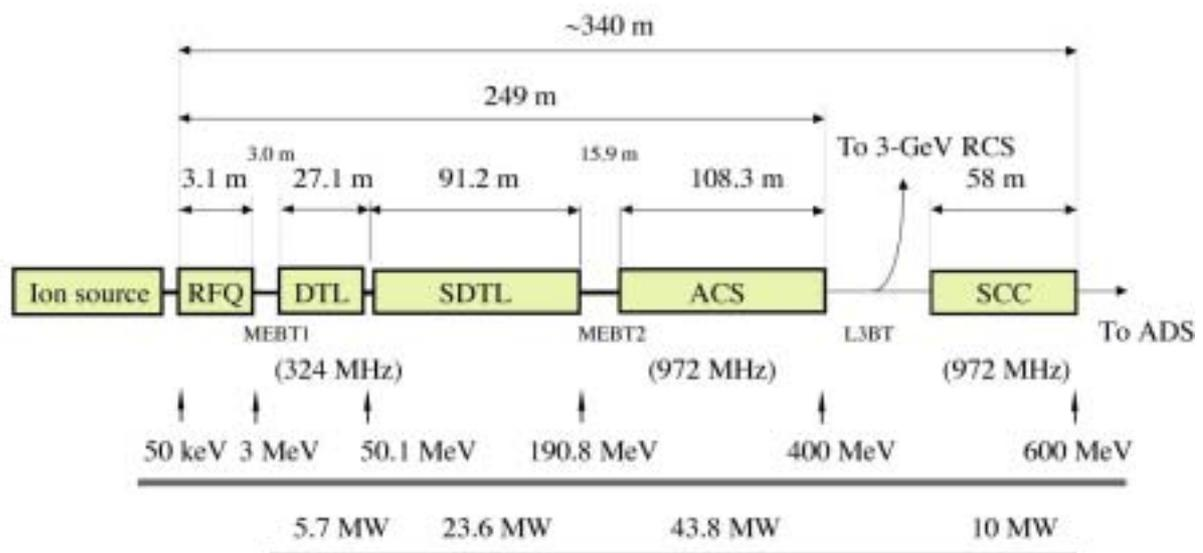
FIG. 1.4: Accelerating scheme of the linac
