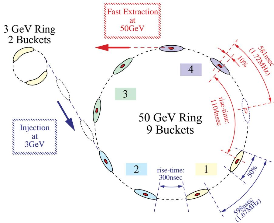
FIG 1.2: Injection scheme from the RCS to the MR
