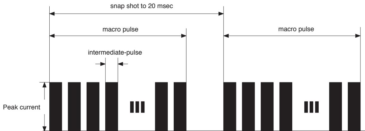
Figure 9.2: Time structure of the linac beam.
